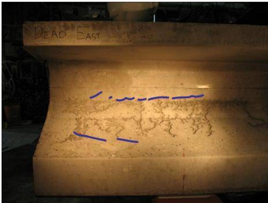
*Figure 4-15: Tx28-I Dead end photo with crack pattern*
