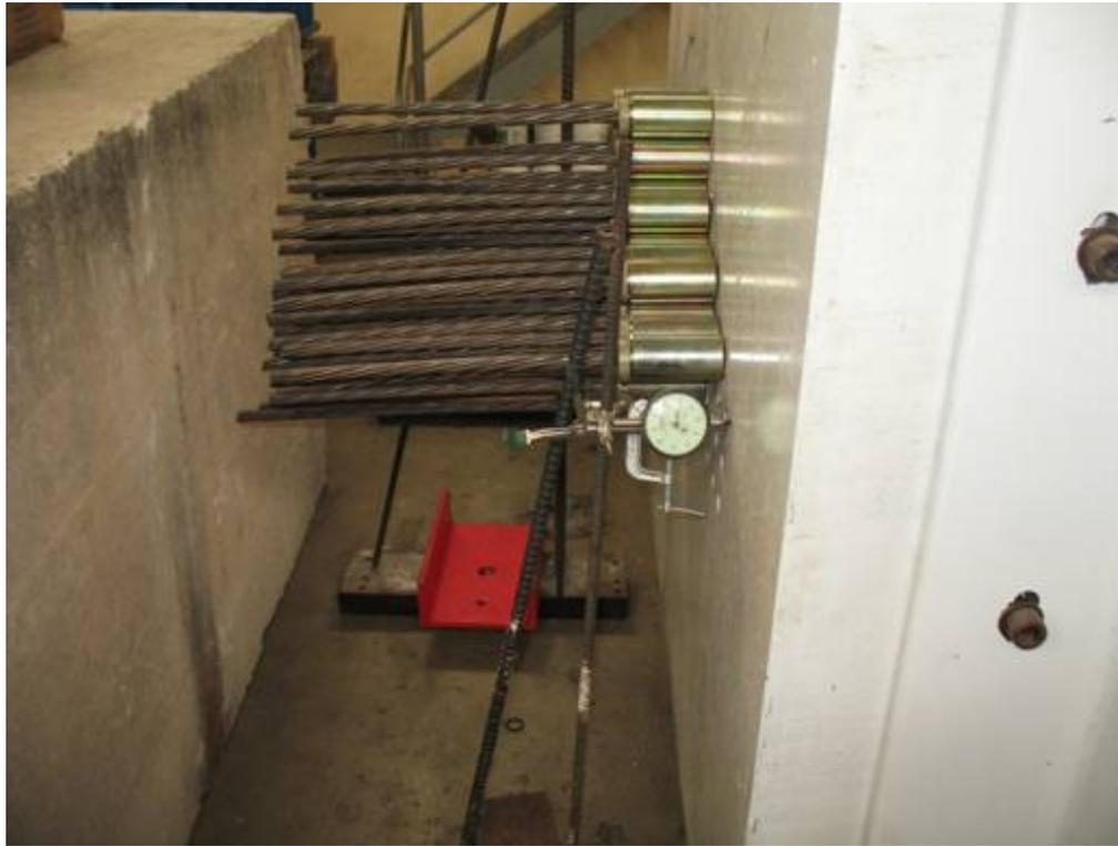
*Figure 3-43: Dial gauges used at dead end of prestensioning bed to measure frame deflection*
