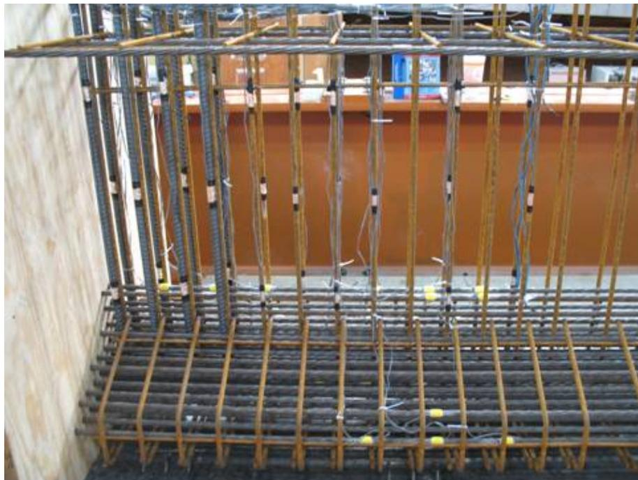
*Figure 3-22: Strain gauges of reinforcing bars and strands*
