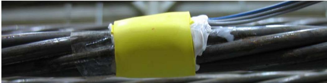
*Figure 3-35: Completed strain gauge on 0.6" diameter strand*
