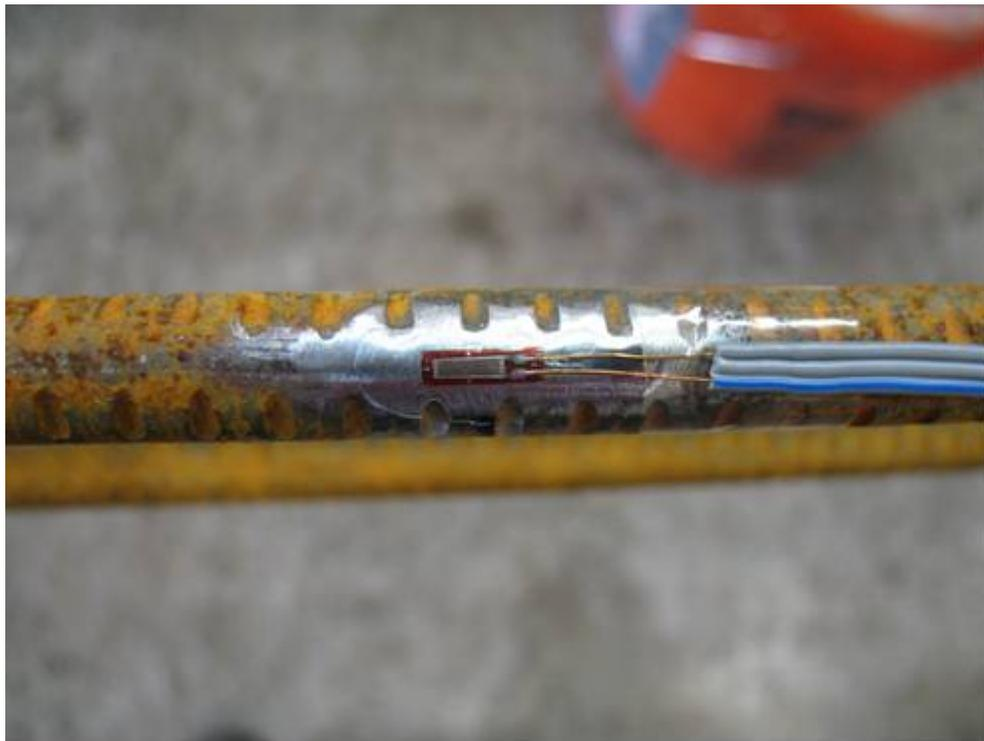
***Figure 3-23: Strain gauge on WWR***
