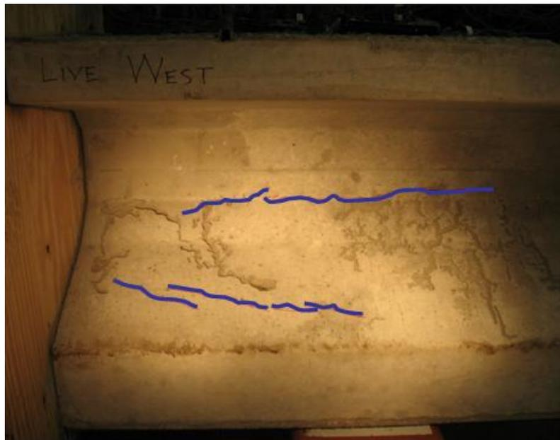
*Figure 4-13: Tx28-I Live end photo with crack pattern*
