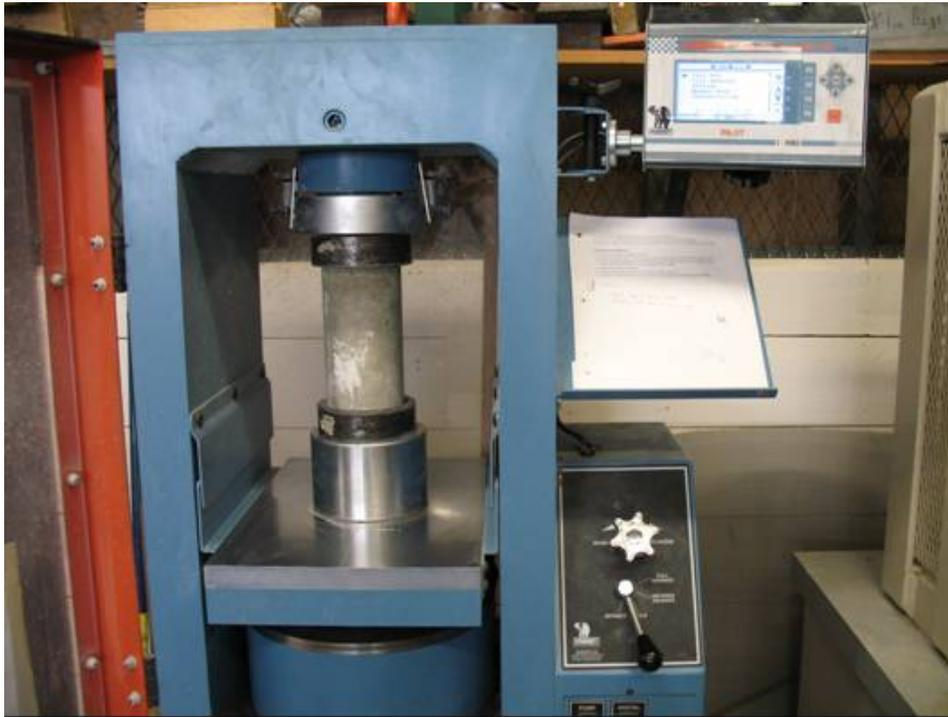
***Figure 3-5: Forney concrete cylinder testing machine***
