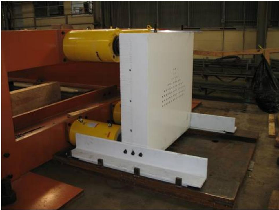
*Figure 3-20: Live end stressing bulkhead with rams*
