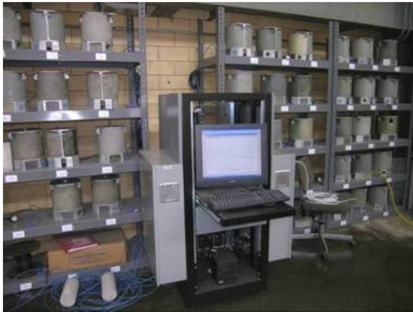
*Figure 3-8: Sure Cure Controller and Cylinders*
