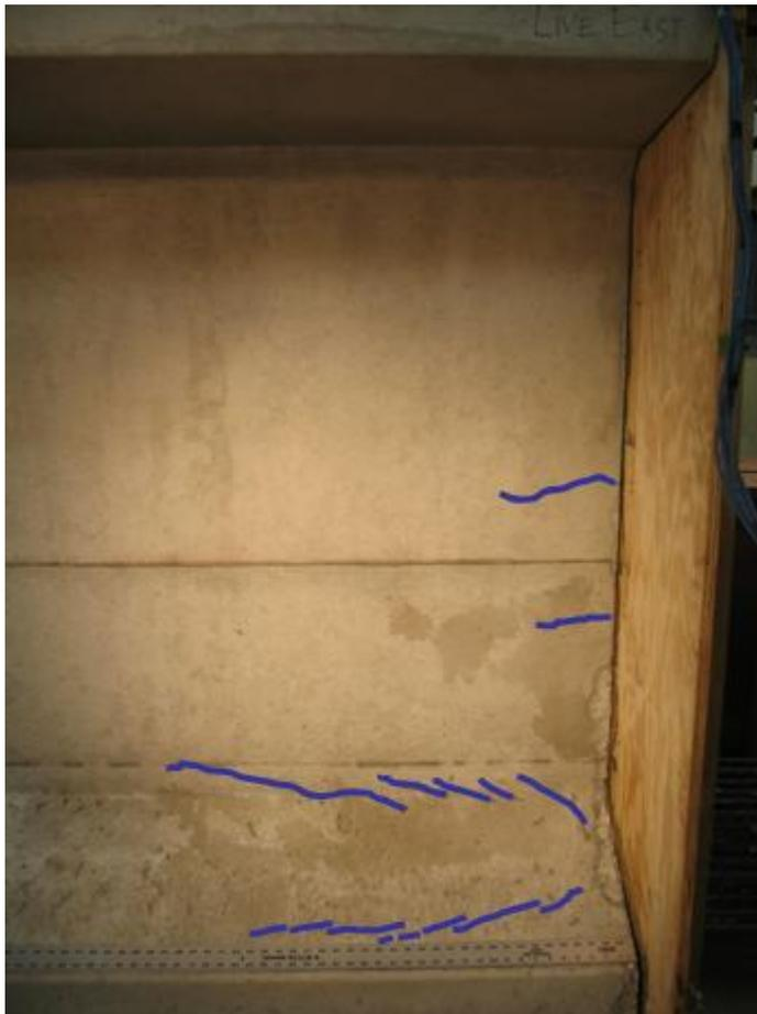
*Figure 4-38: Tx70 Live end photo with crack pattern*
