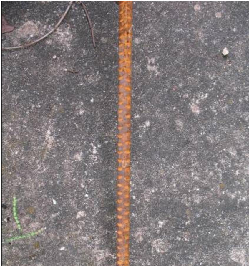
*Figure 3-13: Typical deformed wire from WWR fabrics*
