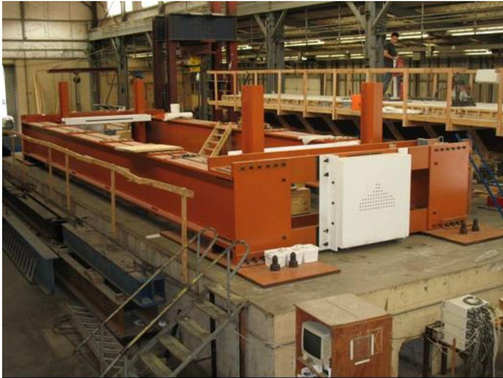
***Figure 3-19: Completed Pretensioning Bed***
