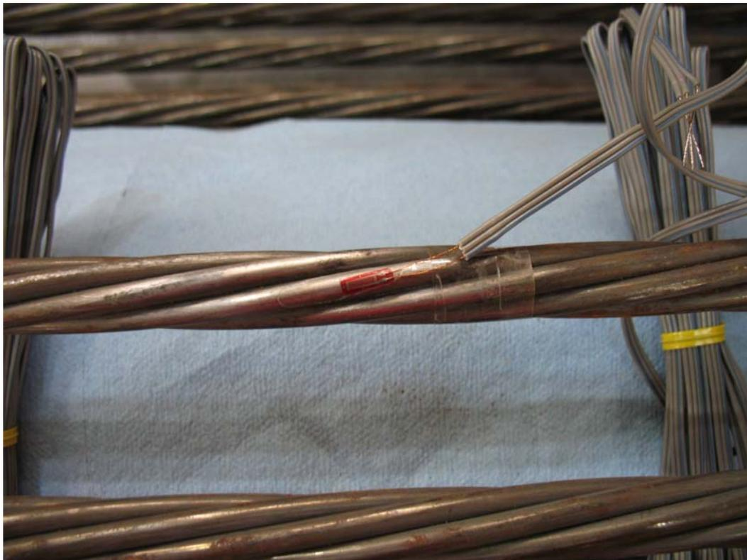
*Figure 3-32: Strain gauge orientation for 0.6" diameter strand*
