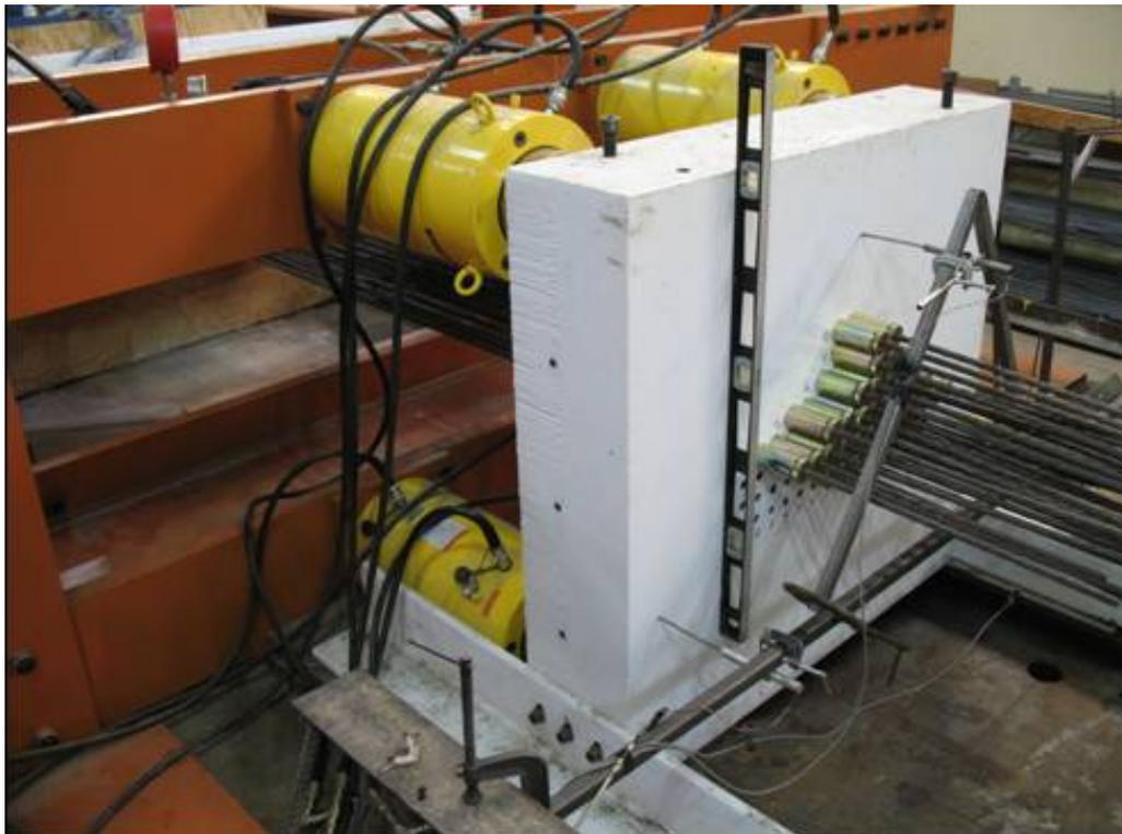
*Figure 3-42: Three Linear Potentiometers measuring strand elongations*
