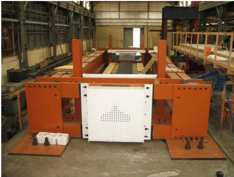
*Figure 3-16: Completed pretensioning bed from dead end*
